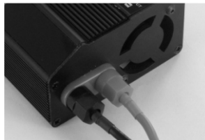
4mm Bullet Connectors plugging to eFUEL power supply directly
