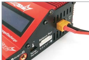
XT60 Connectors plugging to charger directly
